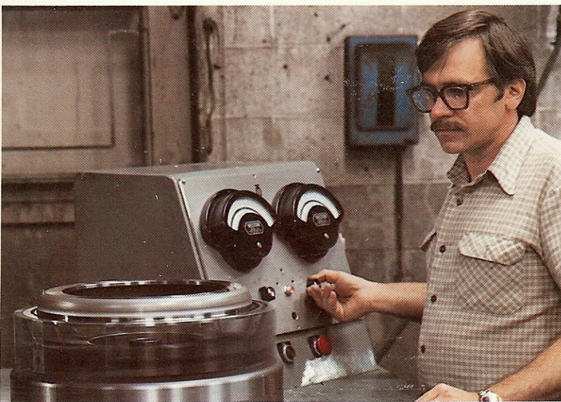
Torque converter parts are checked by spin balancing.
