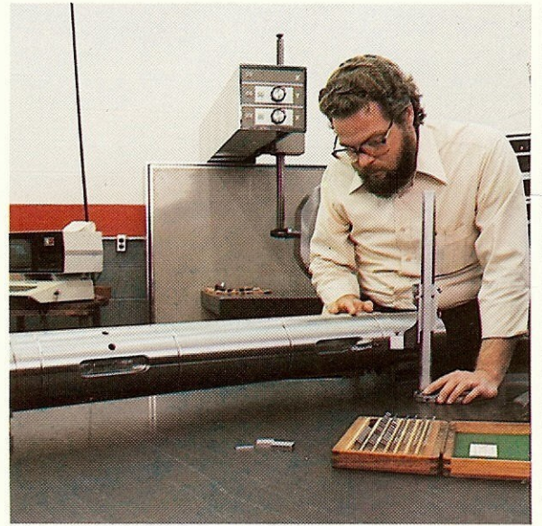
Fairlane's Quality Control department checking keyways on a large pump shaft.
