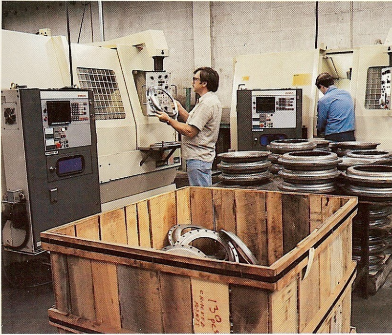
NC lathes used to produce medium-size precision torque converter parts.
