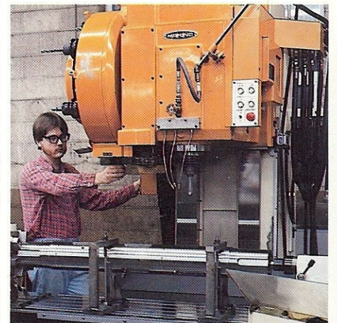
Precision indexed keyways in a large pump shaft are possible by using our 4-axis machining center.
